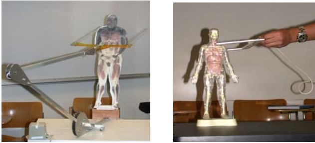
Figure 2: Design A (left) has an adjustable arm, a fork representing the slice plane, and a 2D body. Design B (right) features a 3D body model and free-moving fork.
